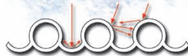
Collector Cross Section showing heat trap design for better all day performance, even on windy days.
